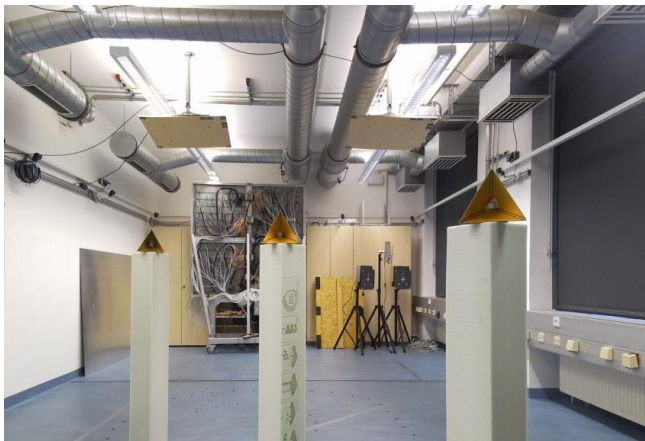
Corner reflectors and Optitrack markers are used for calibration.
