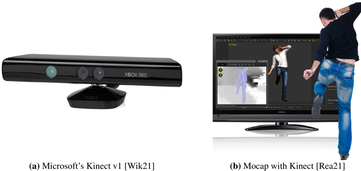
Figure 4.2: Microsoft's Kinect as a human motion capture system.; (a) Microsoft Kinect v1, (b) Mocap with the Kinect.
