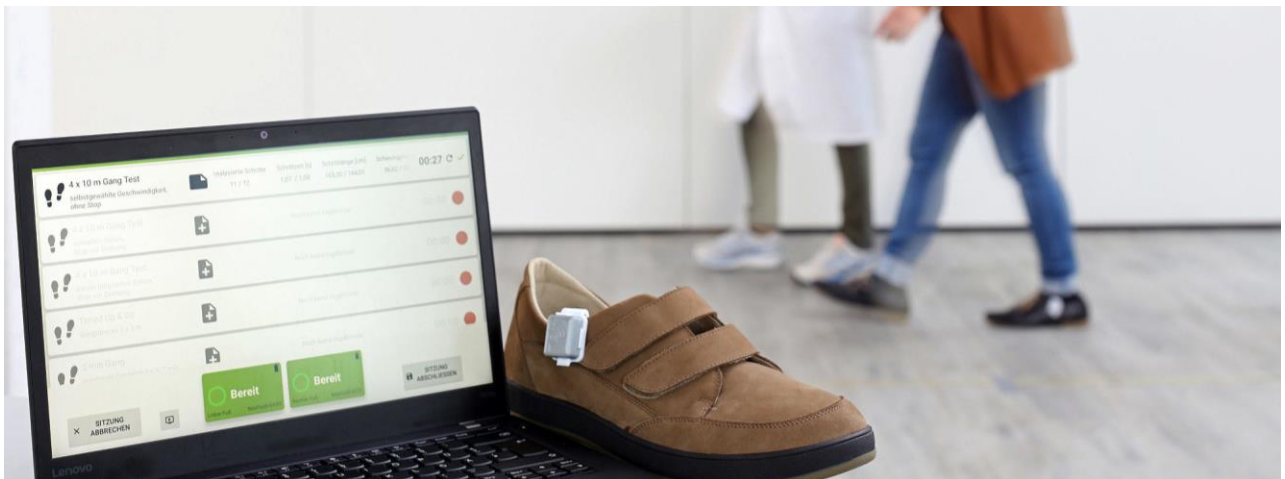
Fig. 1: Gait analysis system with wearable sensors.
