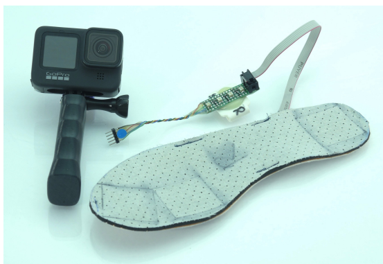
Figure 3.4: Reference system with camera and FSR insole.
