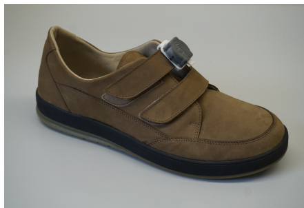
Figure 3.2: Shoe Sensor Placement. The IMU sensors were attached to both feet by mounting them to the shoe as shown.
