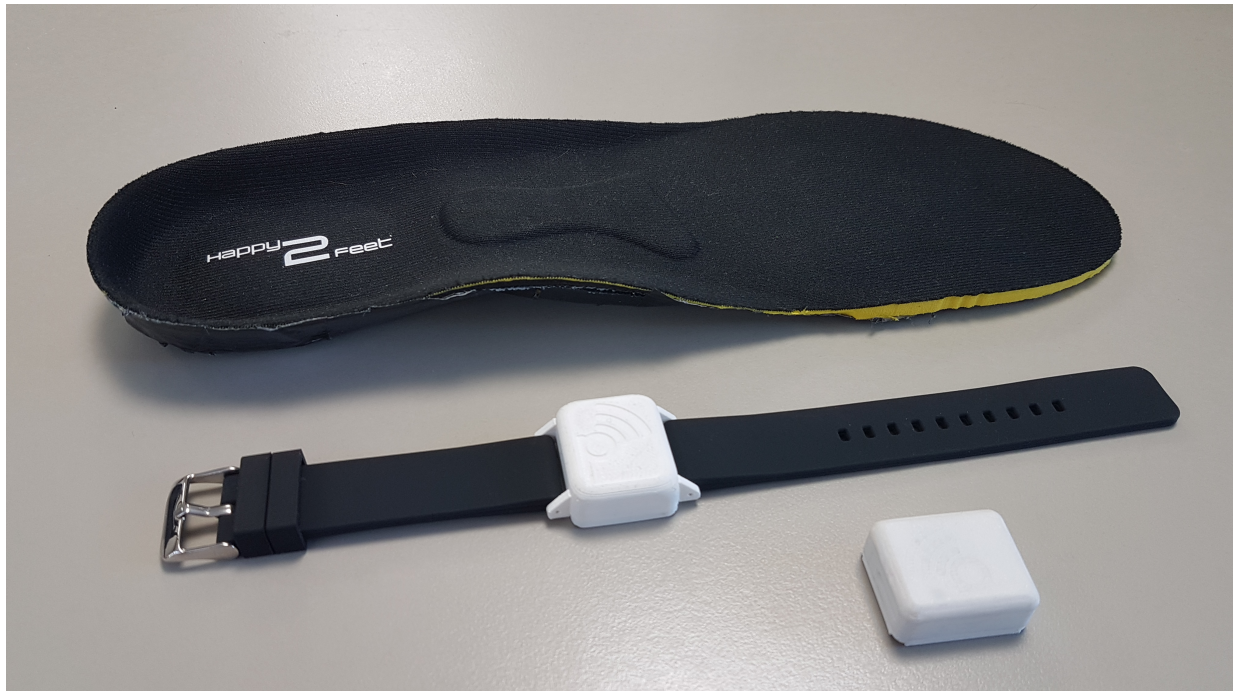
Figure 3.5: The three NilsPod sensor types, Insole (back), Hoop, and classic NilsPod sensor (front) record human movements for healthcare, mobility, and sports applications.
