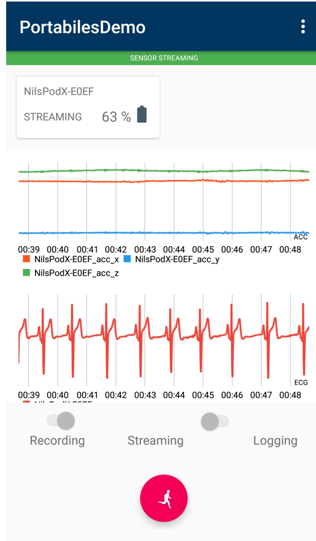
Figure 4.2: Android application for controlling the sensor. Accelerometer data (upper section) and ECG data (lower section) can be streamed in real-time (as depicted in the screenshot) or logged onto the internal sensor storage.
