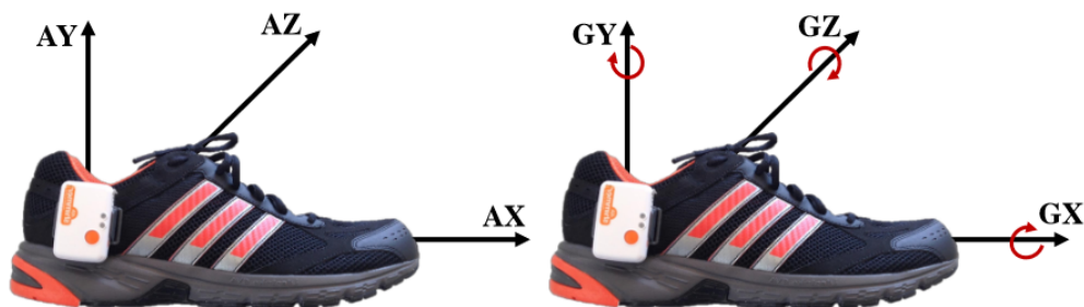
Figure 4.1: Shimmer 2R Sensor. IMU-sensors attached to the shoe and all the signals which are recorded by accelerometer (A) and gyroscope (G) [Bar17].
