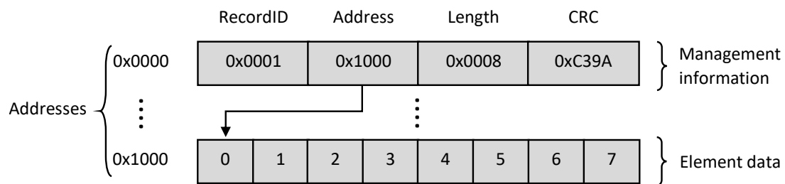
Figure 2.14: Filesystem with management sector. The management information for each data element is separated in a management sector. The management entry references the data element and contains additional information, such as a unique element number, the length of the element and a checksum.
