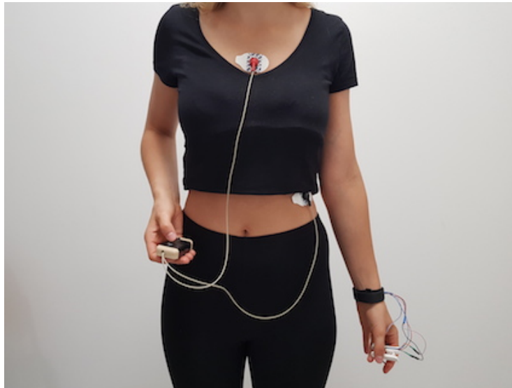
Figure 4.3: Sensor attachment: The ECG sensor is attached with two electrodes, which are placed at the top of the sternum and at the left anterior axillary line. The PPG sensor is attached to a finger on the left hand and connected to the arm position detection sensor unit on the left wrist.
