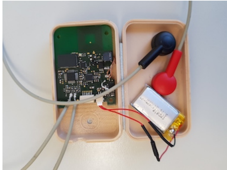
Figure 4.4: ECG sensor: Hardware of the ECG sensor, including the circuit board, the battery and two leads for the electrodes
