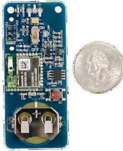
Figure 2.1: Custom Hardware Badges. With a dimension of 3\text{ cm} \times 7\text{ cm} , the badges are small enough to fit in a standard plastic name tag holder and designed to be worn around the neck. Image source: http://www.rhythm.mit.edu/open-badge/
