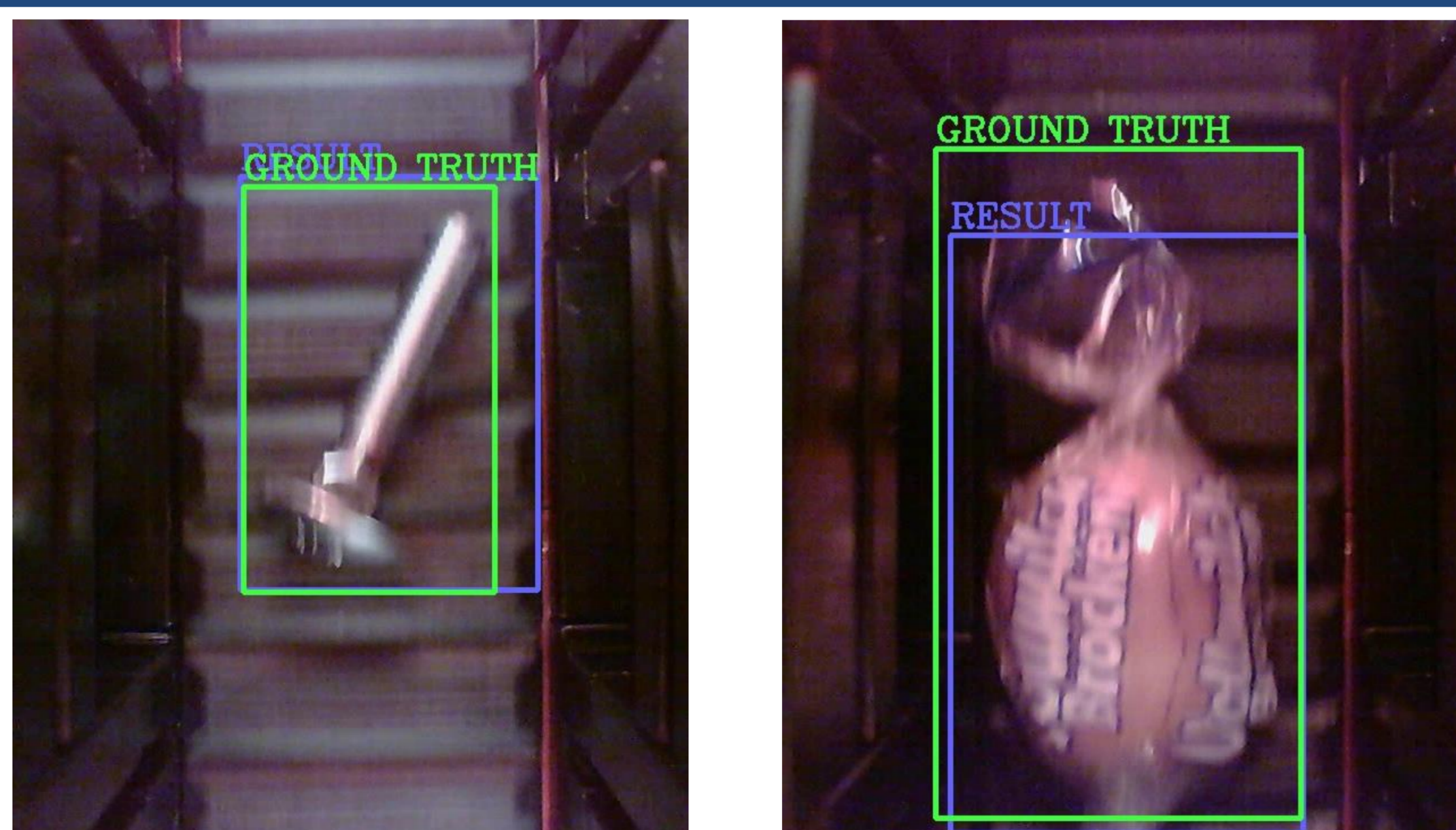
Figure 2: Result of Yolo[5] with screw (left) and candy (right)
